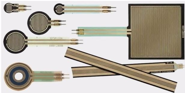
Each sensor has 2 wires which form 1 connector. These can be plugged in the the FSRio on one of the 8 ports, the direction does not matter here.
